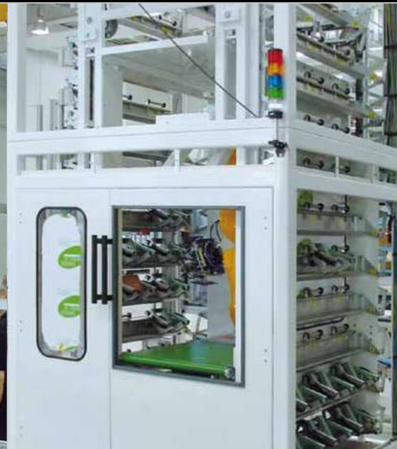
Capacity: 28 carriers Total live load: 1,400 kg [3,086 lb] Carousel dimensions: L 1.70 m [66.9 in], H 3.27 m [10 ft 8 in], D 1.80 m [70.9 in] Carrier dimensions: L 1.20 m [47.2 in], H 0.20 m [7.9 in], D 0.20 m [7.9 in] Machine type: EM-35-100-247-28-200
