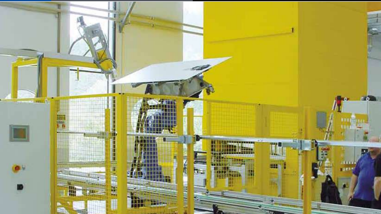
Capacity: 20 carriers Total live load: 2,600 kg [5,732 lb] Carousel dimensions: L 2.75 m [9 ft], H 5.60 m [18 ft 5 in], D 2.60 m [8 ft 6 in] Carrier dimensions: L 2.10 m [82.7 in], H 0.36 m [14.2 in], D 1.08 m [42.5 in] Machine type: EM-75-500-406-20-1080 Controller: ERP interface
