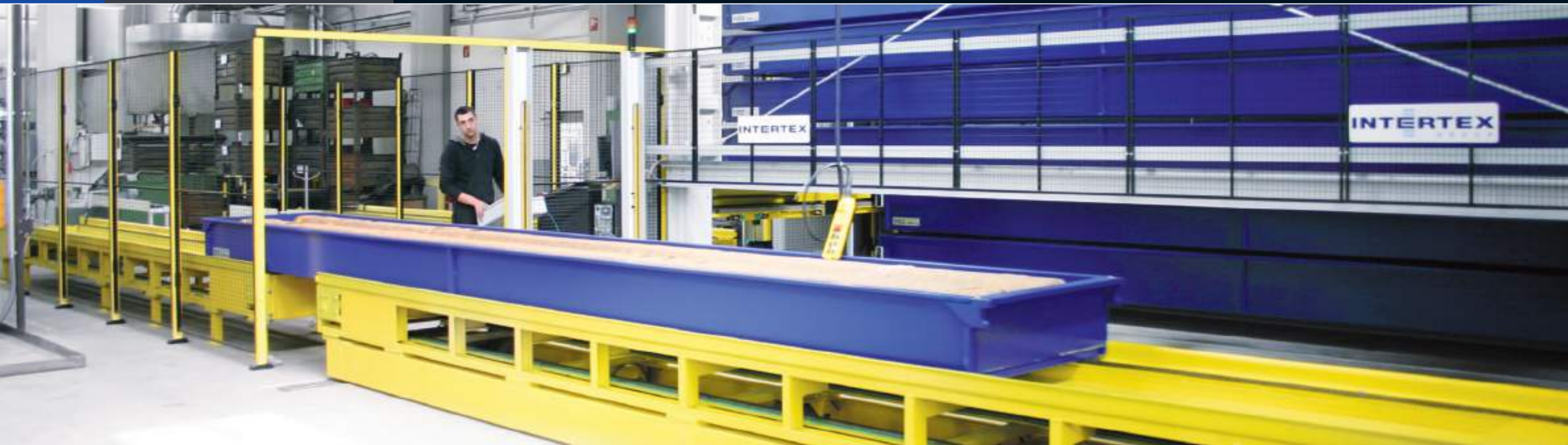
The cassettes are transferred out onto a delivery table with a chain conveyor via a loading cart with chain conveyor.
