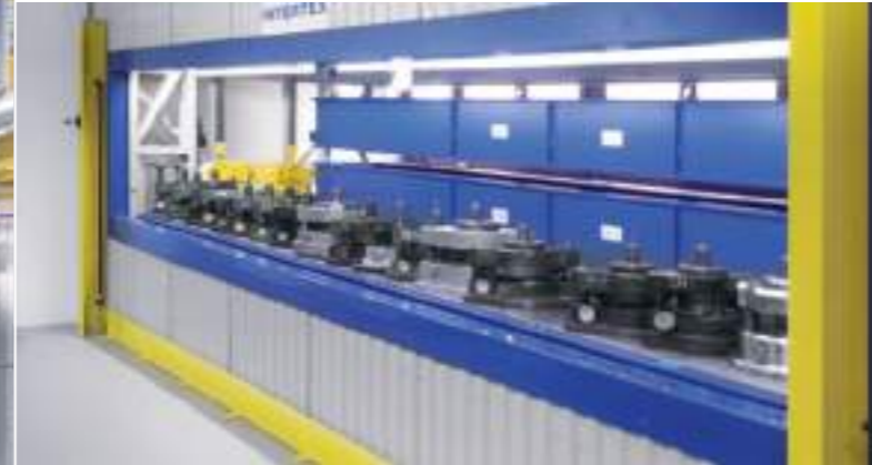
Capacity: 26 cassettes / L 6,000 mm, D 520 mm, H 420 mm Payload per cassette: up to 4,000 kg Machine dimensions: H 9,160 mm, W 7,000 mm, D 2,100 mm
