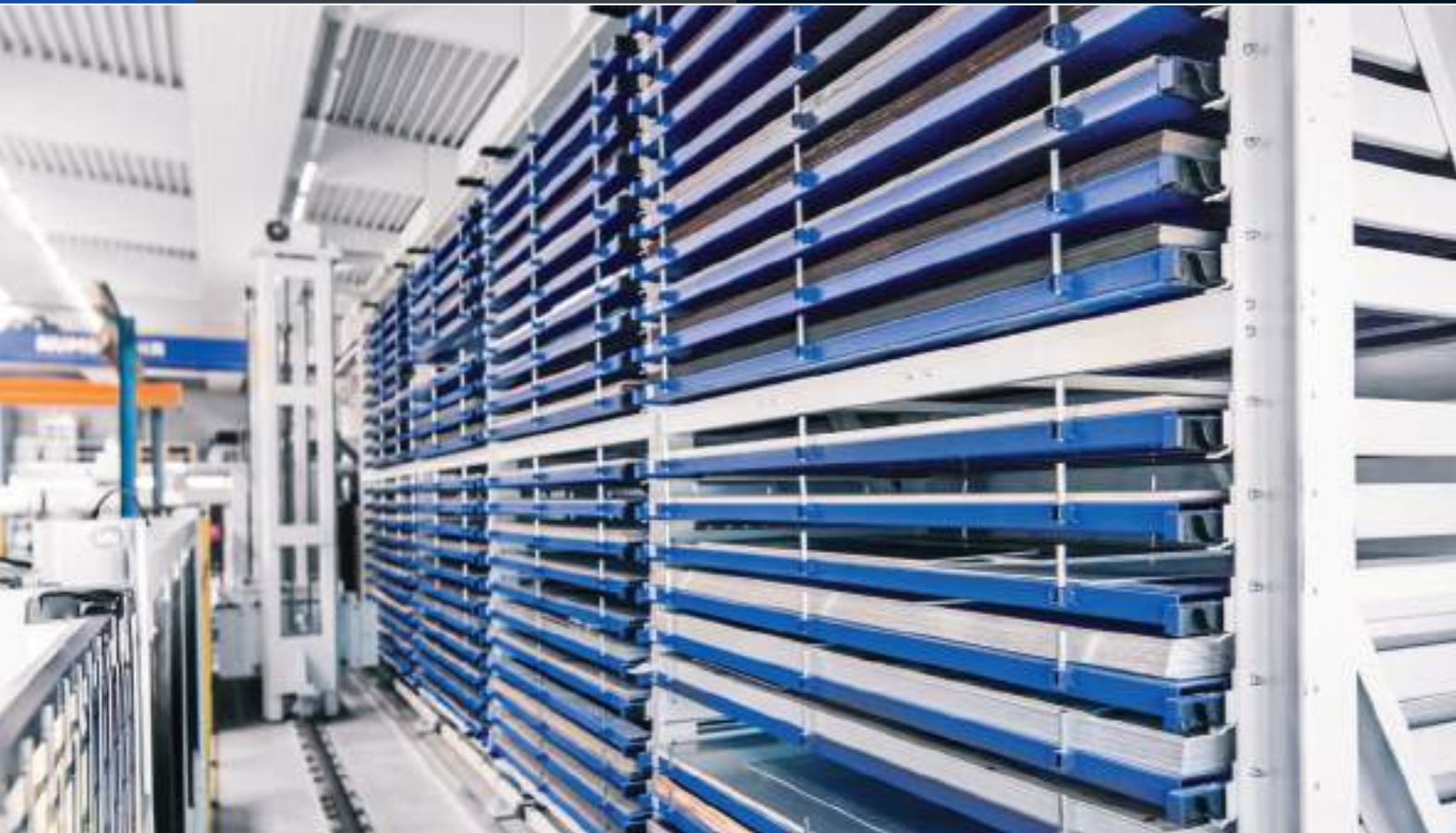
Capacity: 84 pallets / L 3,100 mm, D 1,540 mm, H 90 mm Payload per pallet: up to 3,000 kg Machine dimensions: H 5,515 mm, W 18,900 mm, D 6,200 mm
