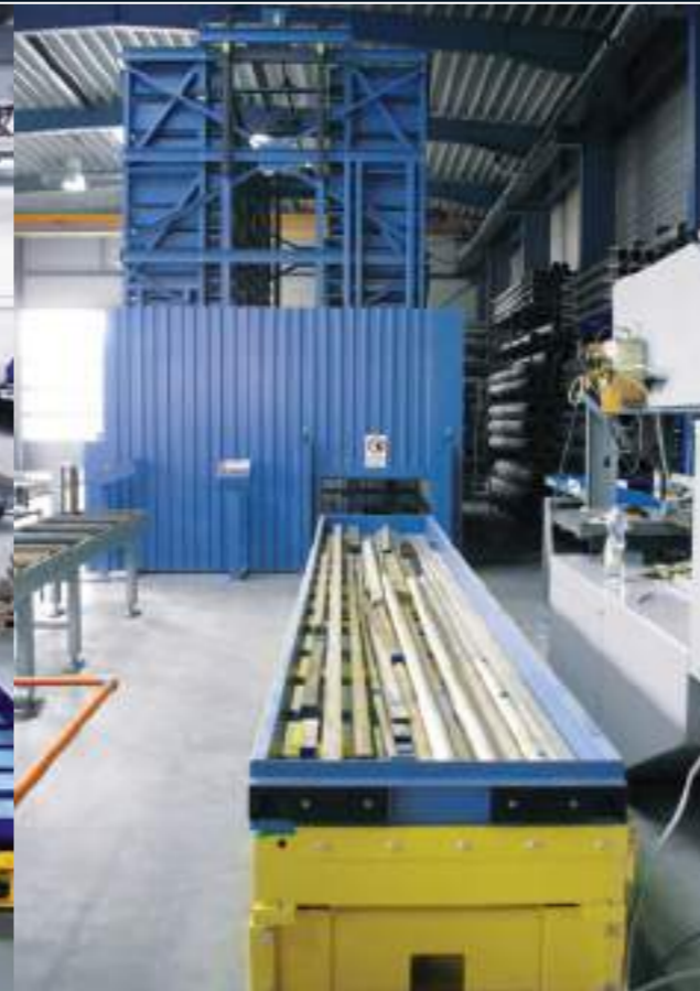
Capacity: 32 cassettes / L 6,500 mm, D 800 mm, H 150 / 300 mm Payload per cassette: 3,000 kg Total payload: 96,000 kg Machine dimensions: H 5,400 mm, W 7,460 mm, D 3,330 mm
