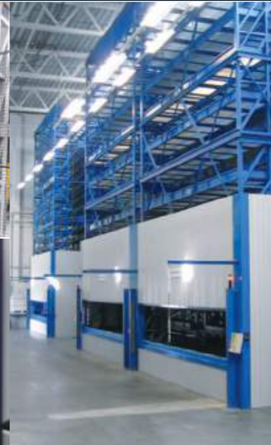
Capacity: 24 cassettes / L 6,300 mm, D 830 mm, H 500 / 830 mm Payload per cassette: up to 2,000 kg Machine dimensions: H 12,700 mm, W 7,260 mm, D 3,330 mm
