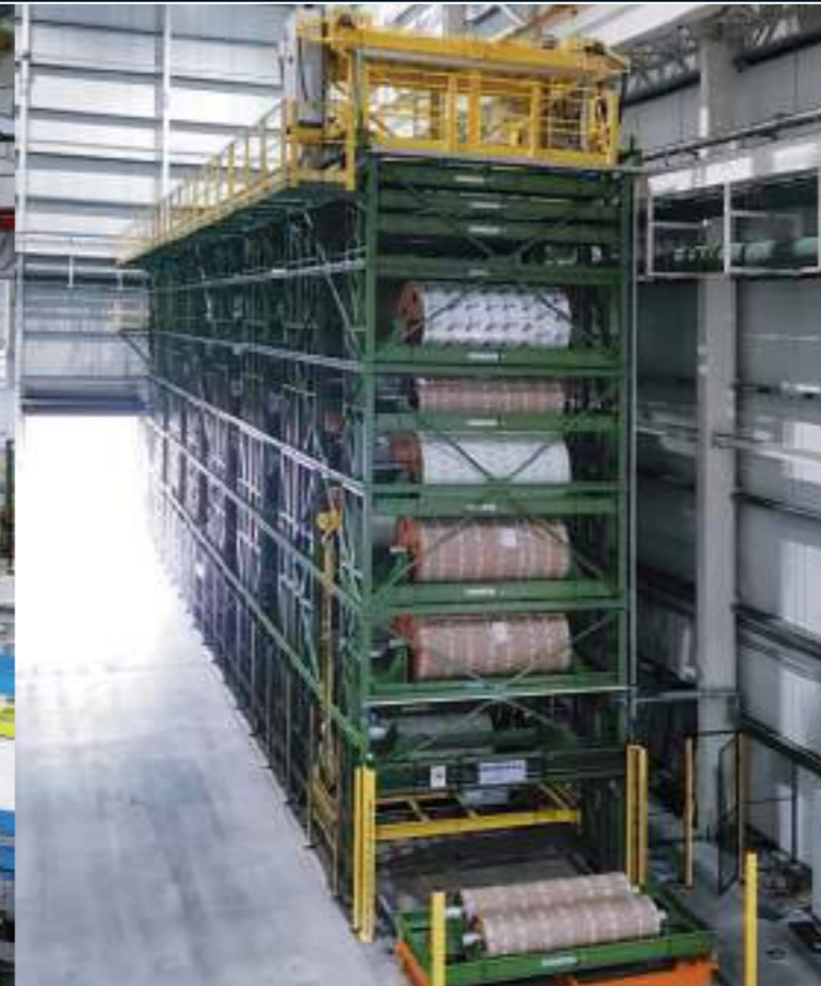
Capacity: 145 cassettes / (250 rolls) / L 3,600 mm, D 1,220 mm, H 300 / 600 / 800 / 1.200 mm Payload per cassettes: up to 5,300 kg Machine dimensions: H 14,000 mm, W 5,400 mm, D 30,000 mm
