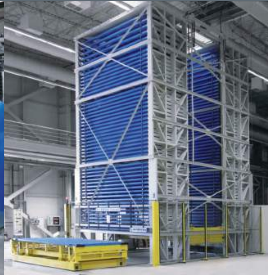
Capacity: 102 pallets / L 4,100 mm, D 2,100 mm, H 50 / 130 mm Payload per pallet: up to 1,500 kg Machine dimensions: H 10,050 mm, W 5,245 mm, D 7,450 mm
