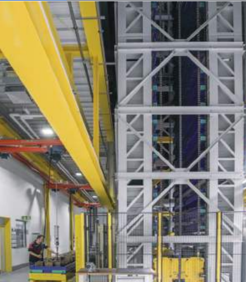
Capacity: 61 cassettes / L 3,500 mm, D 800 mm, H 240 / 480 / 640 mm Payload per cassette: up to 5,000 kg Machine dimensions: H 20,500 mm, W 4,500 mm, D 3,400 mm
