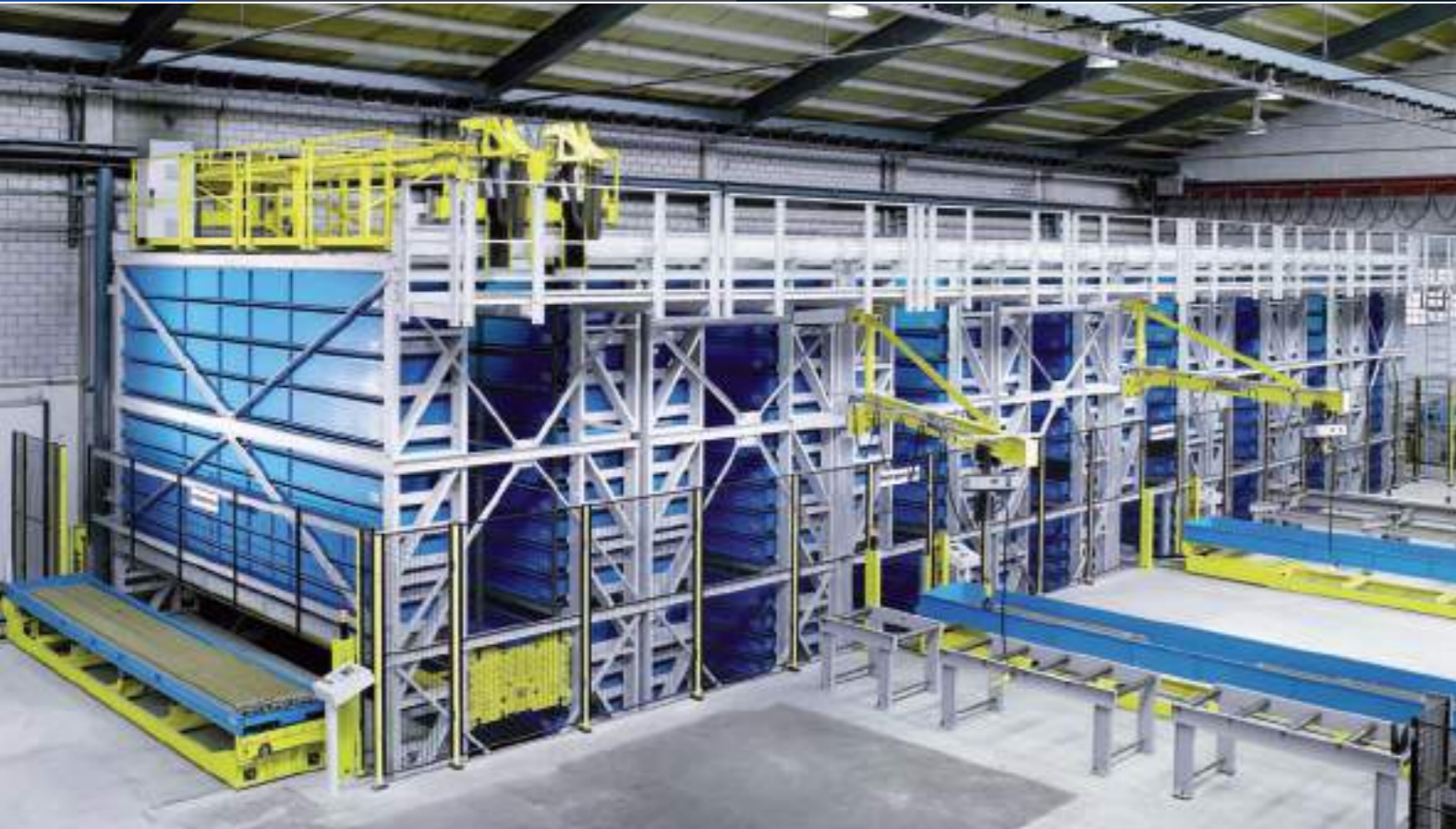
Capacity: 356 cassettes / L 6,800 mm, D 832 mm, H 150 / 200 / 250 / 350 mm Payload per cassette: 3,000 kg / Total payload: 1,068,000 kg Machine dimensions: H 9,140 mm, W 8,900 mm, D 26,000 mm Brüttsch & Rügger Metals AG, CH Regensdorf
