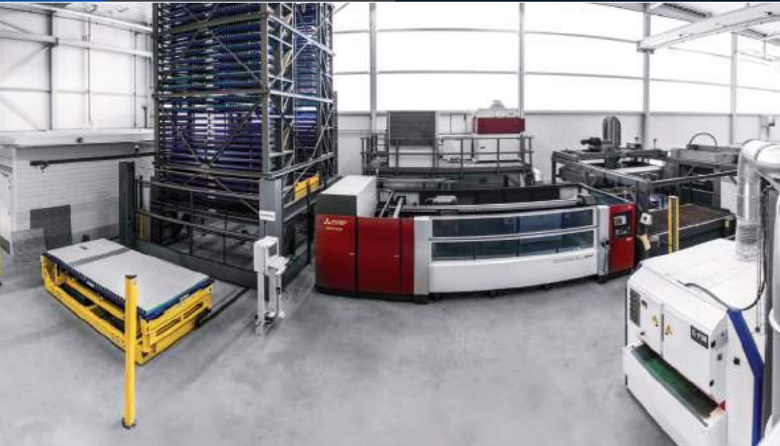
Storage type: TM-FE 2.3 / Storage capacity: 62 pallets Outputs: 1x trolley with lifting and lowering station and 1x double material trolley PickMat-3015 / CO2 Laser system
