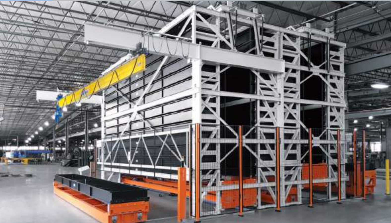
Capacity: 51 cassettes / L 8,100 mm, D 830 mm, H 255 mm Payload per cassette: 1,400 kg Machine dimensions: H 5,615 mm, W 9,000 mm, D 8,850 mm
