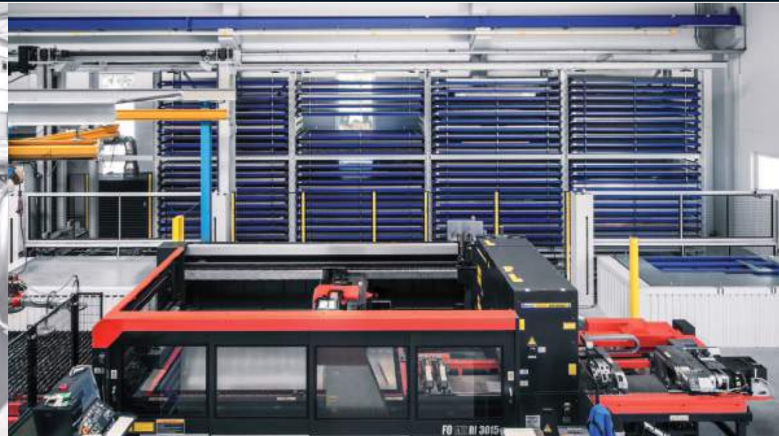
Storage type: TM-RE 4.2 / Storage capacity: 84 pallets Output: 2 x fixed table, 1x with depalletizing station / Vacuum lifter / Laser system
