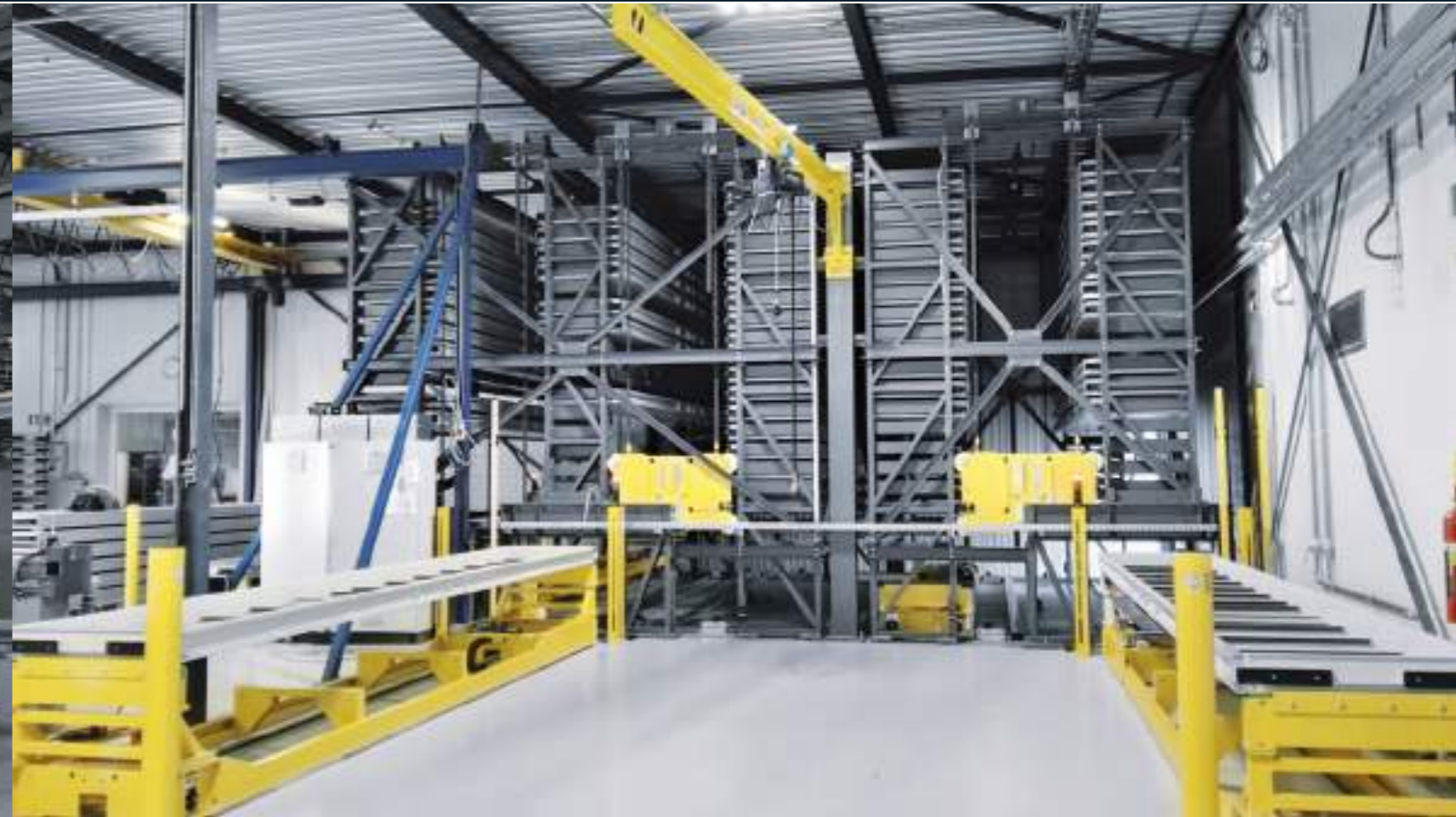
Capacity: 89 cassettes / L 6,300 mm, D 830 mm, H 120 / 150 mm Payload per cassette: 1,500 kg Machine dimensions: H 5,000 mm, W 7,200 mm, D 9,000 mm
