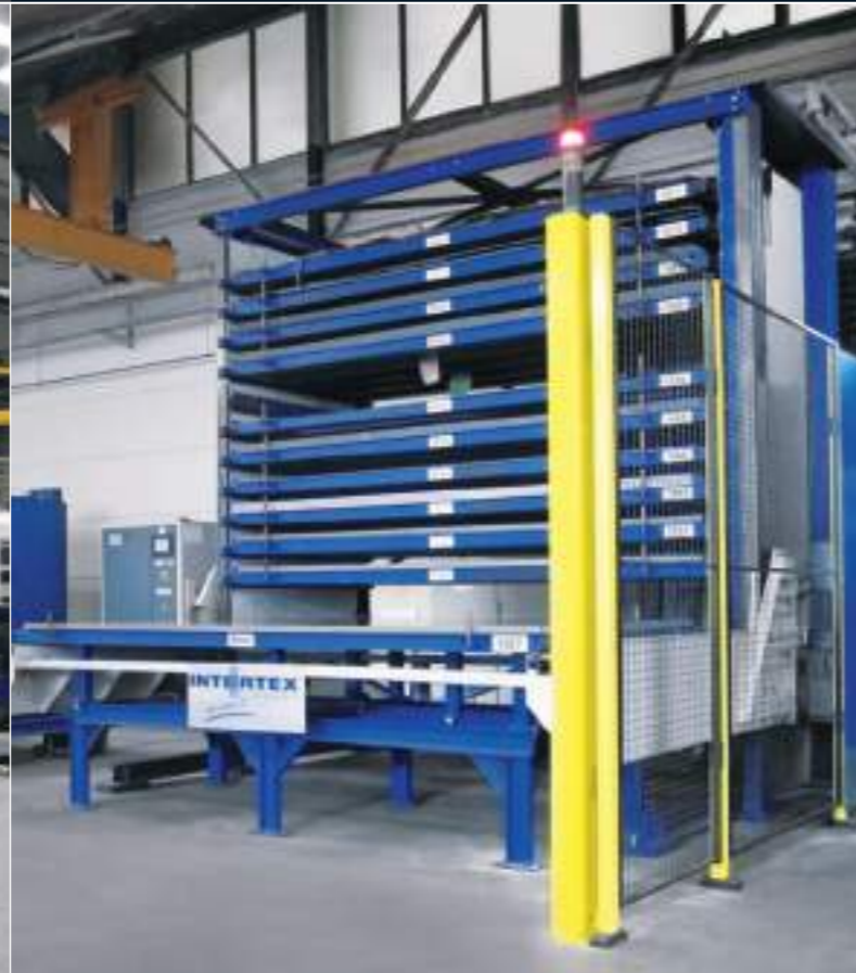
Capacity: 12 pallets / L 3,100 mm, D 1,500 mm, H 90 mm Payload per pallet: 3,000 kg / Total payload: 36,000 kg Machine dimensions: H 3,600 mm, W 4,250 mm, D 3,550 mm
