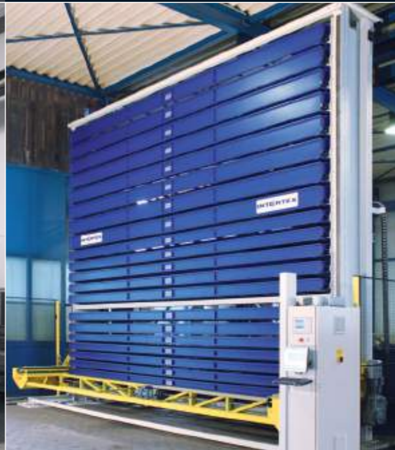
Capacity: 20 cassettes / L 6,300 mm, D 800 mm, H 100 / 150 / 250 mm Payload per cassette: 2,000 kg / Total payload: 40,000 kg Machine dimensions: H 6,225 mm, W 7,200 mm, D 2,200 mm
