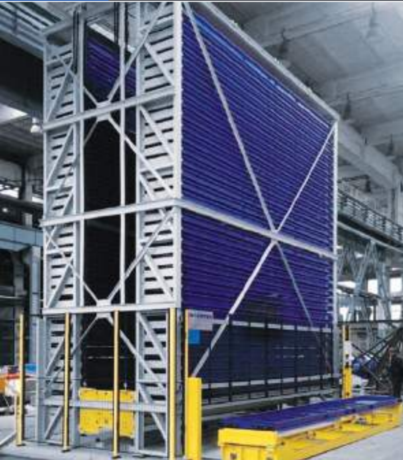
Capacity: 67 cassettes / L 6,300 mm, D 830 mm, H 110 / 150 mm Payload per cassette: 1,500 kg Machine dimensions: H 7,650 mm, W 7,200 mm, D 3,400 mm
