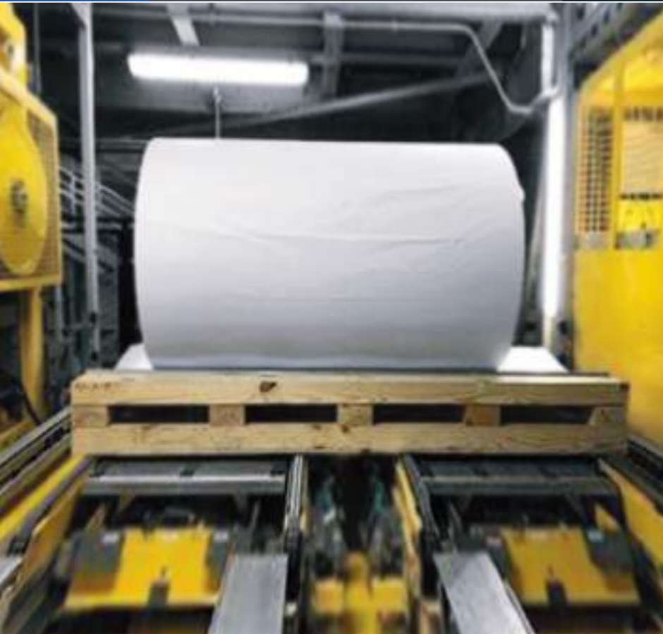
Combination: 2 x 2,5t Paper roll diameter: 1,550 mm Paper roll width: 2,250 mm
