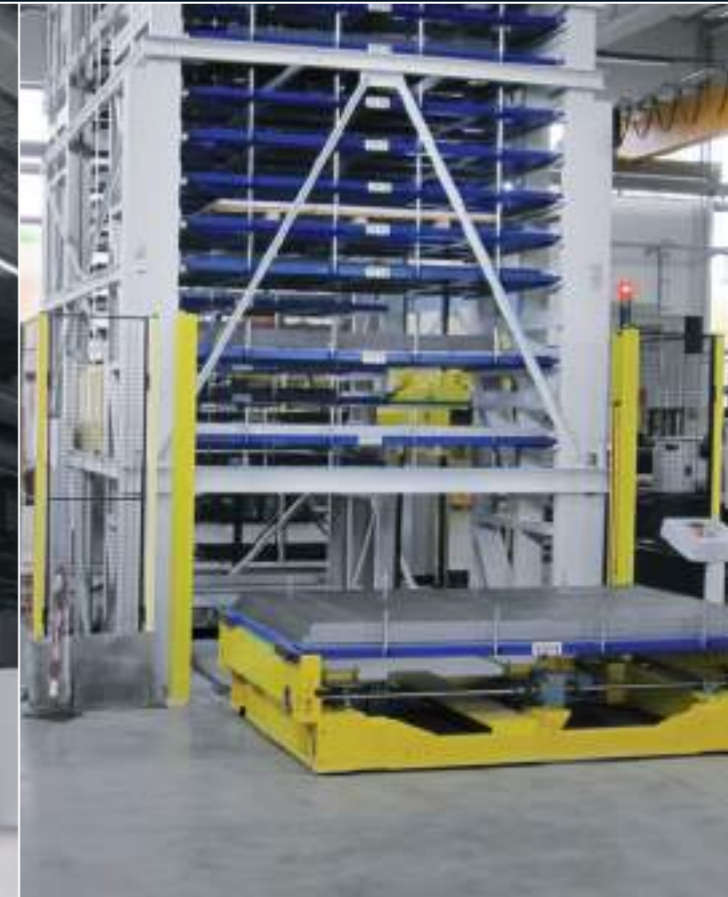
Capacity: 56 pallets / L 2,600 mm, D 1,400 mm, H 120 / 180 mm Payload per pallet: up to 2,500 kg Machine dimensions: H 9,850 mm, W 4,570 mm, D 5,970 mm
