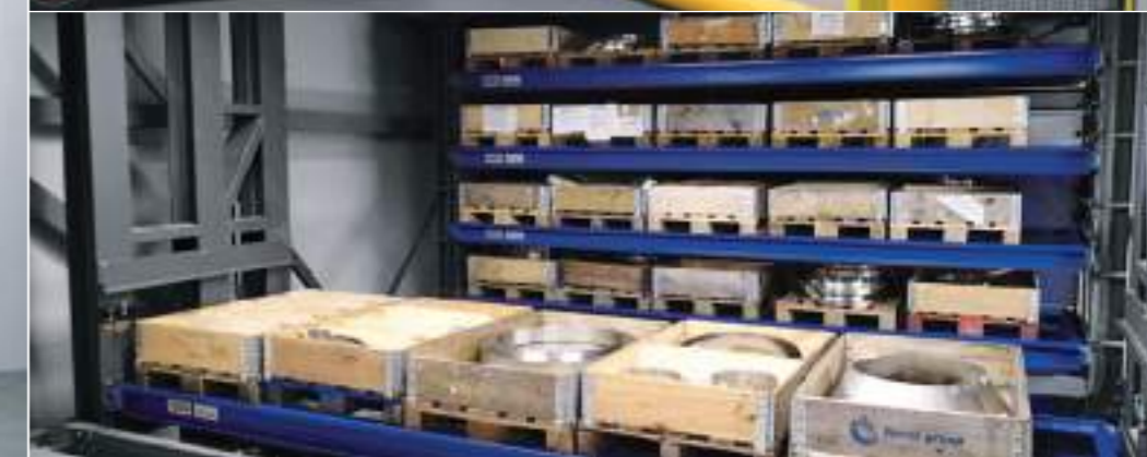
Capacity: 28 cassettes / L 6,000 mm, D 1,300 mm, H 505 / 750 mm Payload per cassette: up to 2,000 kg Machine dimensions: H 10,500 mm, W 6,950 mm, D 6,360 mm
