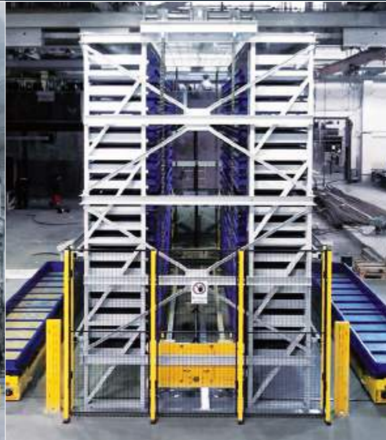
Capacity: 38 cassettes / L 6,300 mm, D 830 mm, H 150 / 200 mm Payload per cassette: 2,000 kg Machine dimensions: H 5,600 mm, W 5,500 mm, D 3,300 mm
