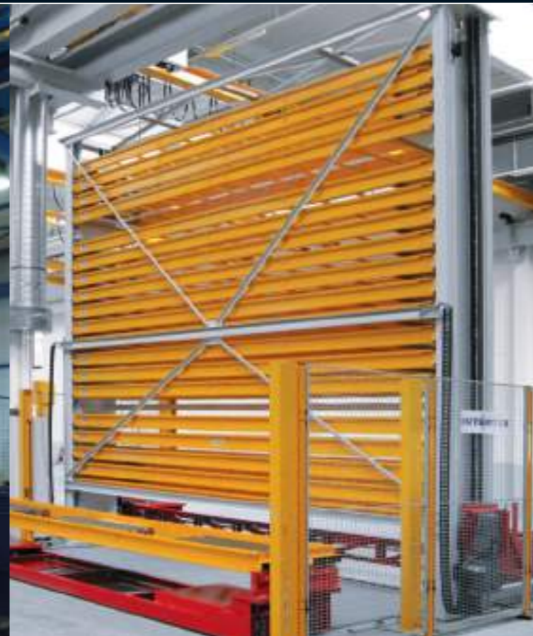
Capacity: 20 cassettes / L 6,300 mm, D 830 mm, H 150 mm Payload per cassette: 1,500 kg Machine dimensions: H 6,150 mm, W 7,800 mm, D 2,500 mm
