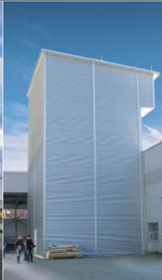
Capacity: 152 cassettes / L 6,300 mm, D 830 mm, H 200-900 mm Payload per cassette: 3,000 kg Machine dimensions: H 15,000 mm, W 8,000 mm, D 12,000 mm
