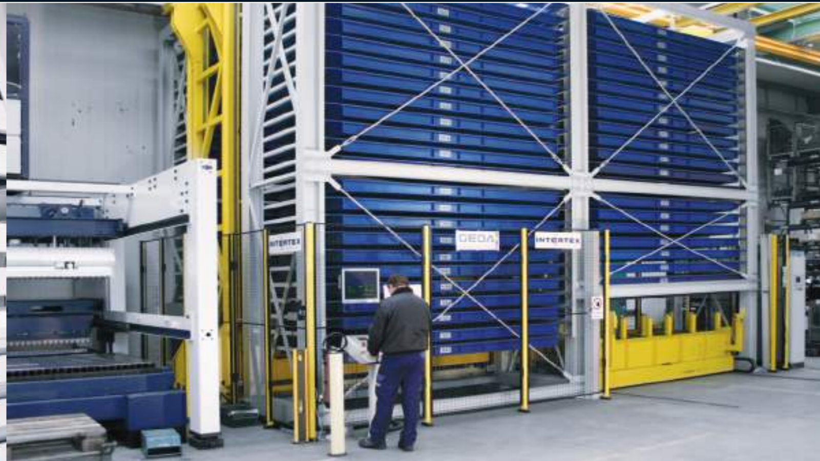
Capacity: 91 cassettes / L 3,100 mm, D 1,600 mm, H 90 mm Payload per cassette: 3,000 kg / Total payload: 273,000 kg Machine dimensions: H 6,150 mm, W 9,870 mm, D 6,130 mm
